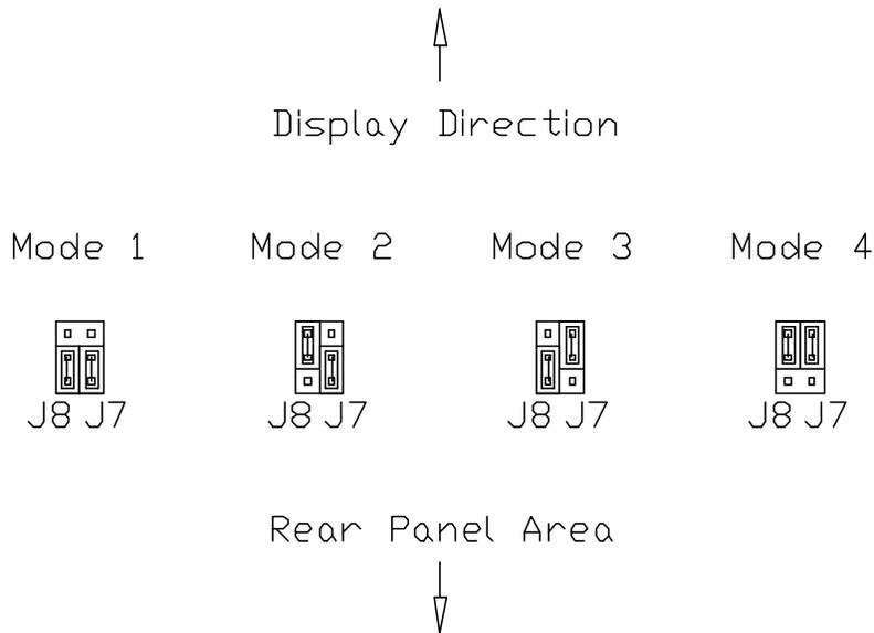
Once the desired mode settings are in place, the top cover of the unit should be replaced, and the screws reinstalled before applying power to the unit. Operation of the unit in the desired mode may be confirmed by observing the DMX Sync indicator lamp, which will blink from 1 to 4 times when power is first applied to the unit to indicate which mode is currently selected.
