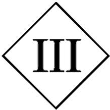
The BL-48 unit provides protection meeting the requirements for Class III electrical products. The unit is intended for operation with external power supplies which comply with the SELV (Safety Extra Low Voltage) requirements. Operation of the unit from power sources which do not meet the SELV standard is not recommended, and may result in an increased risk of electrical shock.
