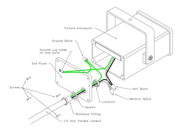
With the AC circuit disabled, remove the insulation to expose about  $\frac{1}{2}$  inch of the bare conductor for each supply wire. Connect the AC supply wires to the AC input lead wires installed in the fixture, following the usual color standards, (Green = Ground, White = Neutral, Black = Hot). These connections can be made using wire nuts, insulated crimp connections, or insulated screw terminal blocks, as available, or as required by local electrical codes.
