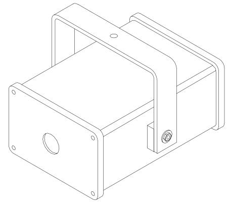
Once installed, the fixture should provide years of service with little or no maintenance required. An occasional inspection of the fixture housing for any evidence of water intrusion, and periodic cleaning of any excessive dirt or dust accumulation on the output window are the only maintenance work recommended.
